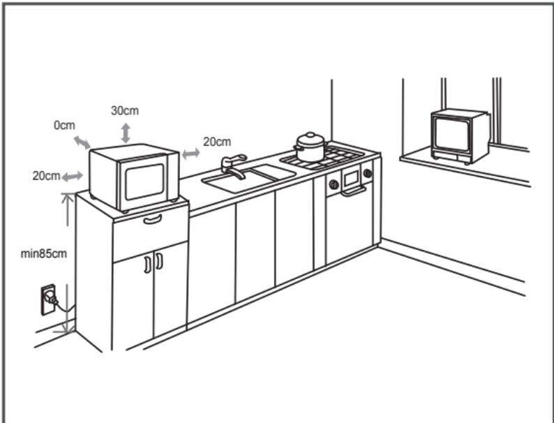
Select a level surface that provides enough open space for the intake and/or outlet vents.
