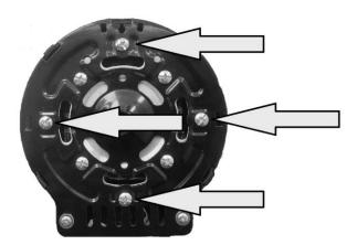
NOTE: Do NOT undo the TIGHT screws – as these hold the motor in place.
